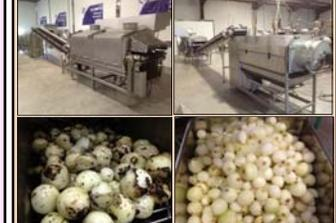
Unitherm Food System Inc. "Flame Peeler & Pasteurizer" tandem equipment process. Top left: same onion; top right: scrubber; bottom left: onions after flame oven; bottom right: onions after oven and scrubber.
