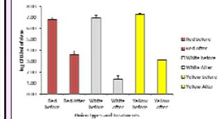
**Figure 4.** Level of *L. innocua* on onions before, and after, processing through the Flame Peeler and Pasteurizer Oven. Data bars represent the means and errors bars represent standard deviation; all trials were done in triplicate replication.
